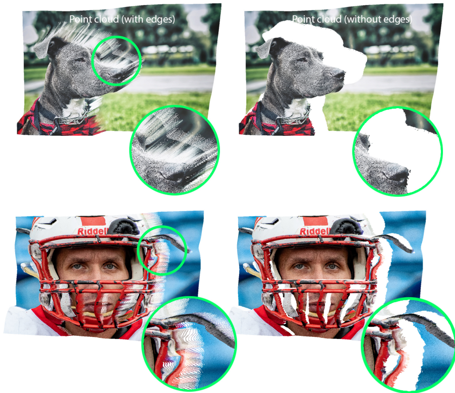
Figure 8.3: Overview of the project point clouds from our high-resolution metric network with and without removal of the high gradient edges that create floating pixels in the 3D space.
