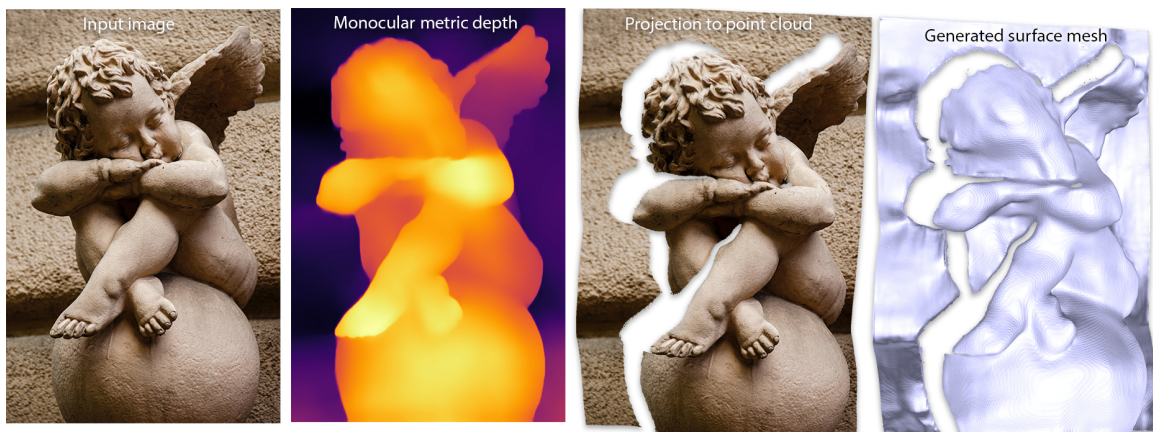
Figure 6.1: The depth estimation from our metric depth network on a photograph in the wild. Our depth estimation is high-resolution with geometric consistency. We can project the metric depth estimation to a dense 3D point cloud. Finally, we can leverage an off-the-shelf meshing network to recover the surface mesh from the 3D point clouds.
