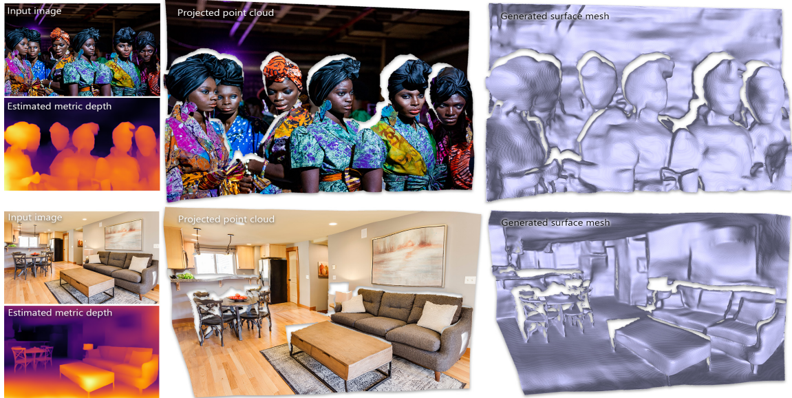
Figure 1.3: We can project our high-resolution metric depth estimations to geometric and coherent point clouds to generate detailed surface meshes from single photographs with varying scene complexities.
