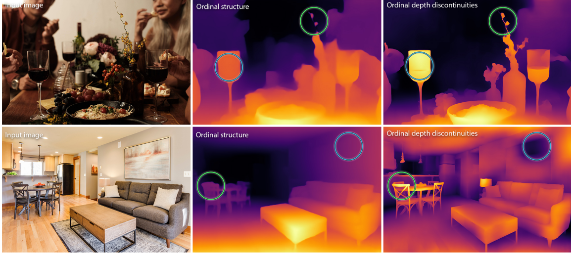
Figure 6.2: Overview of the characteristics of the low and high-resolution ordinal estimations. The low-resolution ordinal estimates capture the scene structure (green circles) but lack high-frequency details (blue circles). On the other hand, the high-resolution ordinal estimates are good at generating sharp depth discontinuities (green circles) but lack structural consistency (blue circles).
