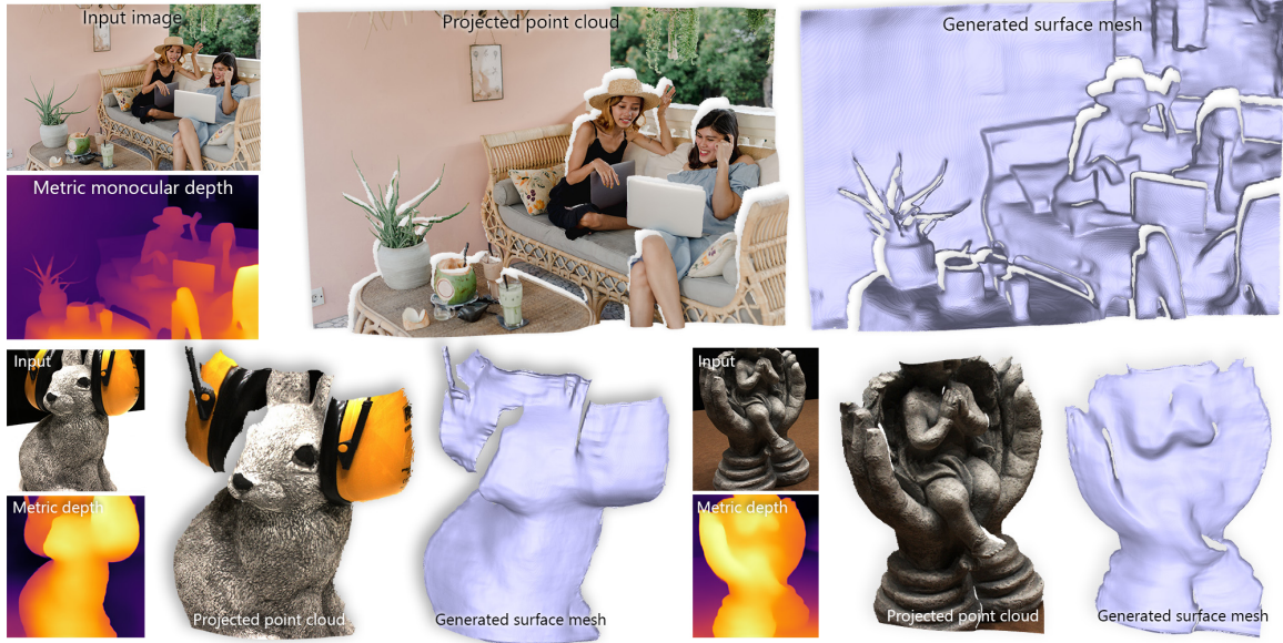
Figure 1.2: Our high-resolution metric depth estimations can be projected to a geometric coherent 3D point cloud to generate detailed surface meshes for complex scenes and single objects.
