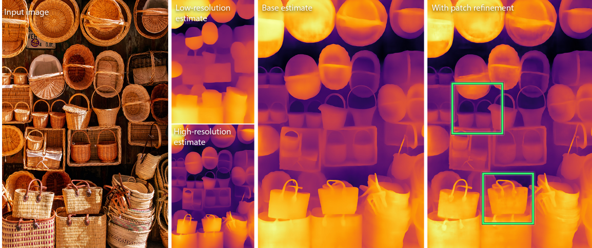
Figure 3.5: Overview of the depth estimation pipeline from boosting framework [32] using MiDaS depth network. For a given image, depth estimations at two different resolutions (receptive field size and R_{20} ) capture scene structure and high-frequency details. Then, the merging network combines the two estimations to generate a high-resolution base estimate. To further improve the intricate details in the base estimate, a patch refinement approach is employed at the image patch level, as seen in the green squares.
